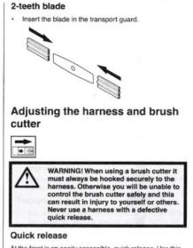
At the front is an easily accessible, quick release. Use this if the engine catches fire or in any other emergency situation that requires you to free yourself from the machine and harness.
