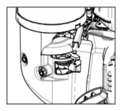
♦1.2Turn the choke lever to the "CLOSE" position
