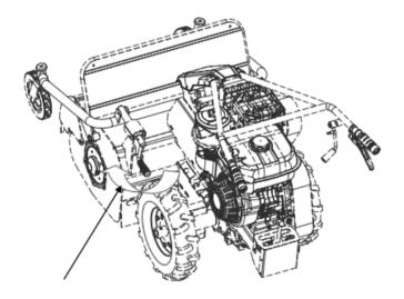
Rotate the height adjustment handle to adjust the clearance between the blade and the ground
