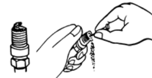
Removal of carbon deposition
