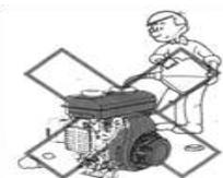
4. Do NOT cover the Engine when in operation!
