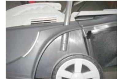
Lock the handle in the position shown, with the supplied screws.
