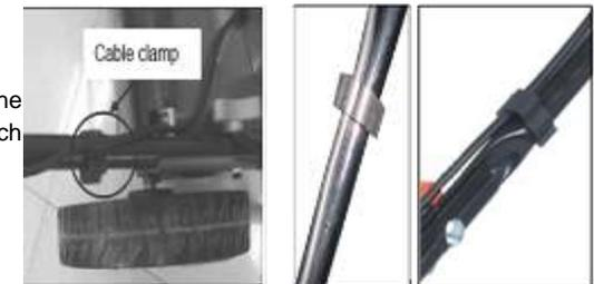
Attach the cable-clamp to the position shown and then attach the cable
