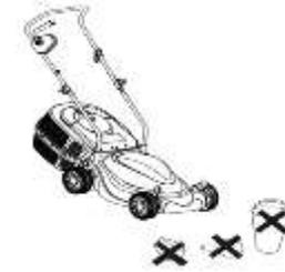
4. Never lift the rear of the mower while starting the motor or during normal operation
