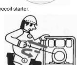
c. Start: Hold recoil starter handle bar and pull it until resistance is felt and then pull the rope rapidly
