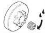
(1) Needle bearing (2) Sprocket (3) Spacer (4) Clutch
